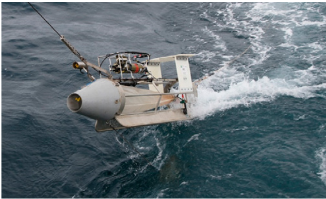
Figure 4: Gulf VII plankton net just after it has been pulled out of the water. The grey conical nose cone with net can be seen at the front. The equipment for measuring salinity, temperature and depth is located in the middle of the frame. At the end of the gear is a white wing that provides stability.
